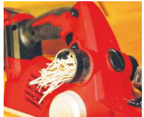
▲ The dust outlet is easily overwhelmed when making wider cuts with the bag fitted
